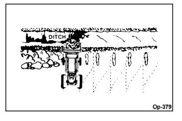
Pile dirt on high side for easier backfilling on a slope.
